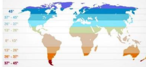
Optimal angle for fixed solar panels depending on installation position.
